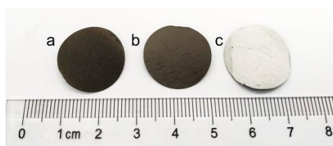
Figure S2 Optical images of NC/GF separator before and after air plasma treatment. (a) NC/GF separator before air plasma treatment. (b) The front side of NC/GF separator after air plasma treatment. (c) The rear side of NC/GF separator after air plasma treatment. The color of the rear side changes from black to white, confirming the NC species was removed thoroughly on this side.
